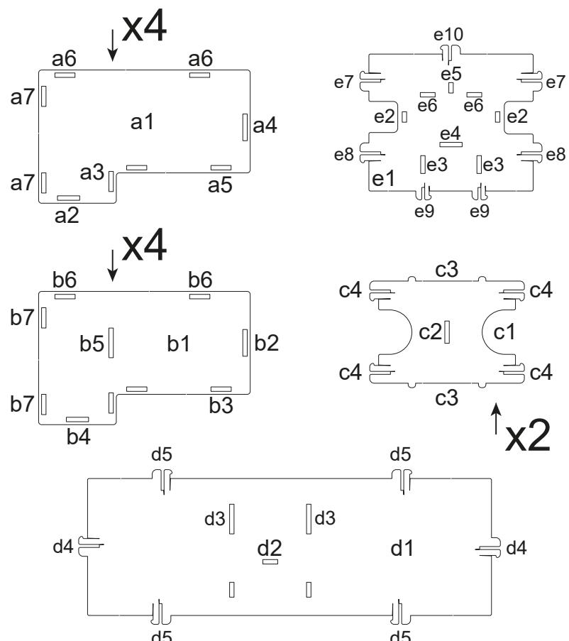
Assemble based on base element letter then according to numbers from first to last.
